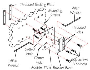
FIGURE | - INSTALLING THE ADAPTER PLATE
